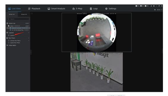
**Step 3:** Right-click the corresponding layout and select Play(P) option to preview the camera in the layout. You can also directly double-click the corresponding layout for quick viewing.
