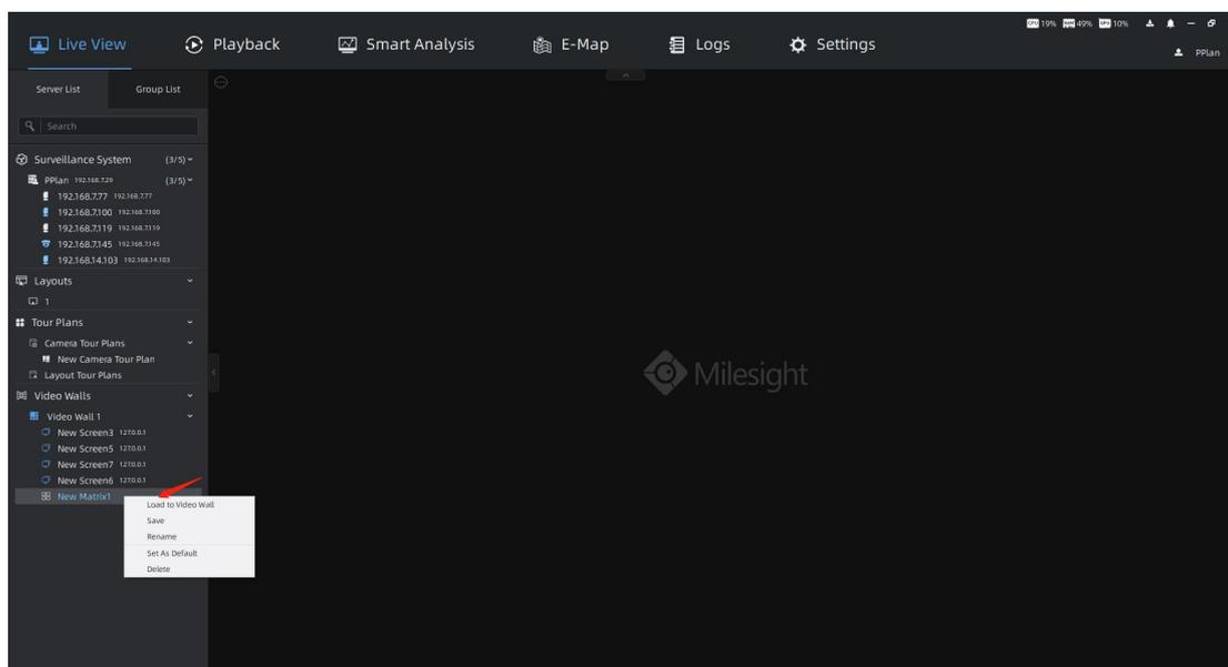
**[Load to Video Wall]:** Each screen will play the content according to the matrix.
