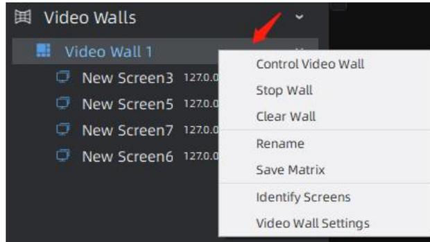
**[Control Video Wall]:** Pop up the Video Wall control window to use the Video Wall.
