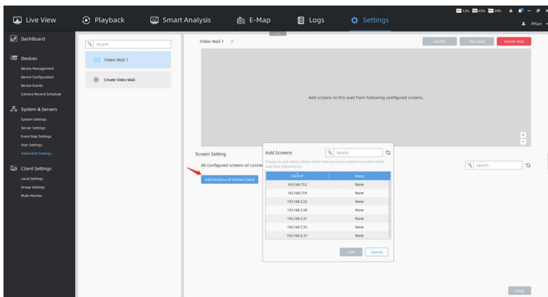
**Step3:** Then select the Client whose screen does not exist in the current Video Wall in the LAN from the list, and click the button **Add**. You can also add multiple Online Clients as needed. Then these added Clients will be displayed in the Screen Setting list. And all monitors actually connected to these Screens will be displayed on the Clients.
