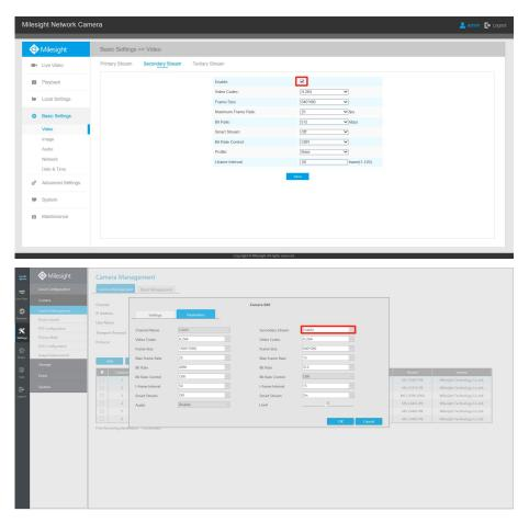
2 For MS-Nxxxx-UT, MS-Nxxxx-UNT and MS-Nxxxx-UPT, please upgrade your NVR to V72.9.0.2-r2 or above, and select Secondary Stream or Primary+Secondary Stream for recording (Primary+Secondary Stream by default.). Then you can select secondary stream for playback.
