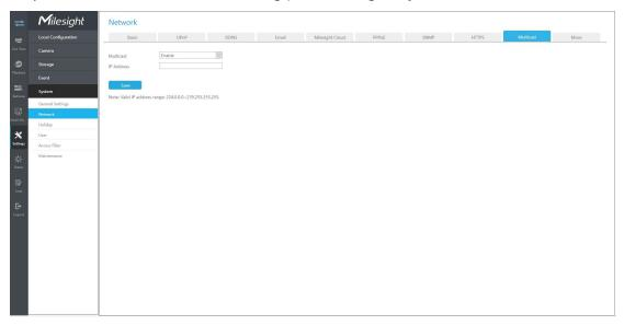
Step2: Configure a multicast IP address for your NVR.
