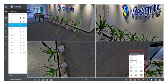
Click icon "Fisheye Client-side Dewarping" to pop up the "Client-side Dewarping" panel. You can set the Installation Mode and Display Mode according to your own needs. For instance, in 103R mode, the viewing angle of R1 image can be adjusted according to the corresponding color border (red) . For more information about the Dewarping Panel, see Part 4 of this article.
