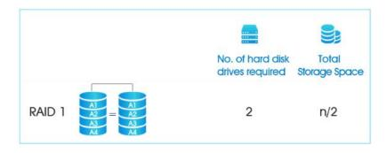
A fault-tolerance configuration known as "disk mirroring." With RAID 1, data is copied seamlessly and simultaneously from one disk to another, creating a replica or mirror.
