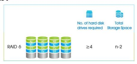
It's identical to RAID 5. Besides, it's an even more robust solution because it uses one more parity block compared with RAID 5. The system is able to normal operation even two disks are dead.
