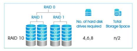
Which is a combination of RAID 1 and 0 and is often denoted as RAID 1+0. It combines the mirroring of RAID 1 with the striping of RAID 0.
