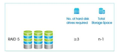
This RAID level provides better performance than mirroring as well as fault tolerance. With RAID 5, data and parity (which is additional data used for recovery) are striped across three or more disks.
