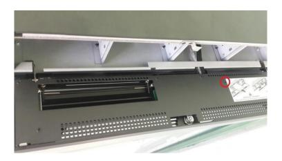
**80XX-UH:** Slide and open the panel, a black button on the inside like the figure shown below.
