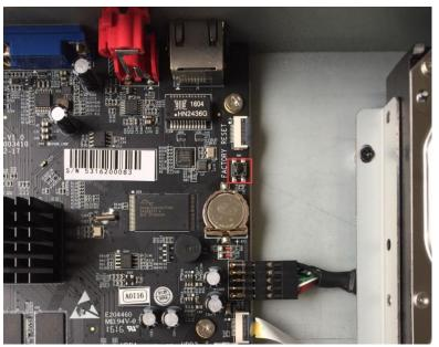
**5008-UPT:** Slide and open the panel, a black button on the inside like the figure shown below.
