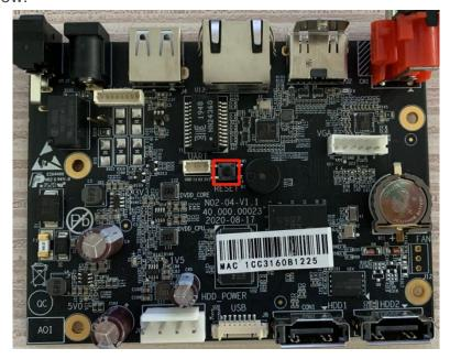
**50016-UT:** Slide and open the panel, a black button on the inside like the figure shown below.
