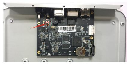
**100X/1009-UT:** There is a hole on the back, use a pin or something like that to push the button deeper inside the hole.
