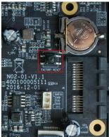
**5008-UPC:** Slide and open the panel, a black button on the inside like the figure shown below.
