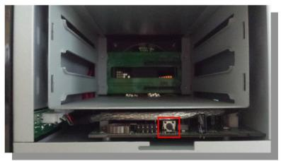
**5008-UC:** Slide and open the panel, a black button on the inside like the figure shown below.
