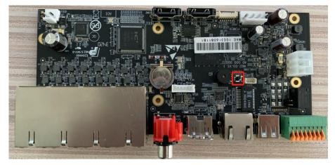
5016-**UPT:** Slide and open the panel, a black button on the inside like the figure shown below.
