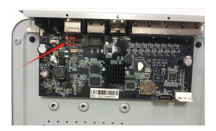
**1009-UPT/UNT:** Slide and open the shell, an orange button on the inside like the figure shown below.
