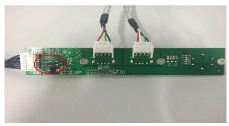
**70XX-UH:** Slide and open the panel, a black button on the inside like the figure shown below.
