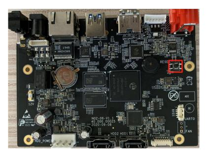
**5016-UH/5032-UH:** Slide and open the panel, a black button on the inside like the figure shown below.
