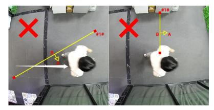
A redundant identification area needs to be left after the target appears in view. This is to ensure that the camera already has stable recognition and tracking of this target when it passes the detection line, which will make the count and detection more accurate.
