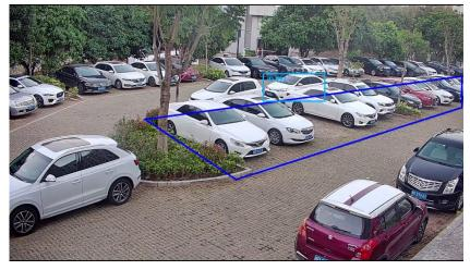
While using Object Left/Removed, there won't be detection boxes. Please try to cover all the objects to be detected. It is recommended that the region is just enough to cover the objects.
