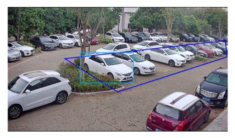
As the following picture shows, when only a small part of the detection box enters the region, the target will not be noted as being in the region.
