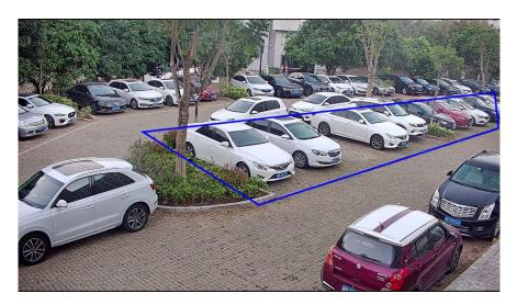
As the following picture shows, when the overlap between detection box and detection region is approximately 80% of the box, the target will be noted as being in the region.
