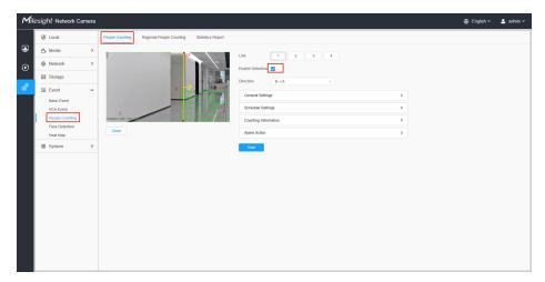
**Step 2:** Draw a line(Up to 4 lines can be set). The direction of the arrow is IN. If necessary, you can also set Min and Max size limits of object to exclude abnormal targets.
