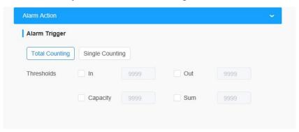
Alarm Action: Configure the specific actions of the camera when the alarm is triggered.
