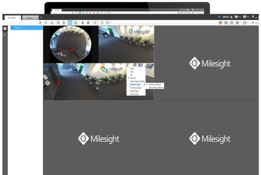
Under Bundle-Stream Mode, it can support Ceiling, Wall, Flat three kinds of installation modes and six kinds of display modes including 10(one Original View), 1P(one Panoramic View), 2P(two Panoramic View), 4R(four Regional View), 1O3R(one Original View and three Regional View), 1P3R(one Panoramic View and three Regional View), to achieve a flexible viewing mode for your demanding. Any of these modes support primary and secondary streams.
