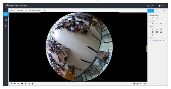
With Multi-Channel Mode, you can set parameters for every dewarping channel.
